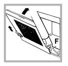
Grip the door on the two external sides and close it approximately half way. Unlock the door by pressing on the clamps **F**, then pull the door towards you lifting it out of its seat (*see diagram*).
